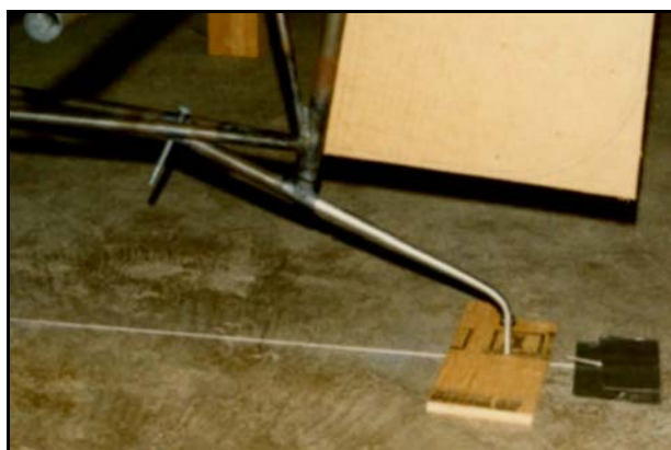
Tailwheel Spring and Support Tube
