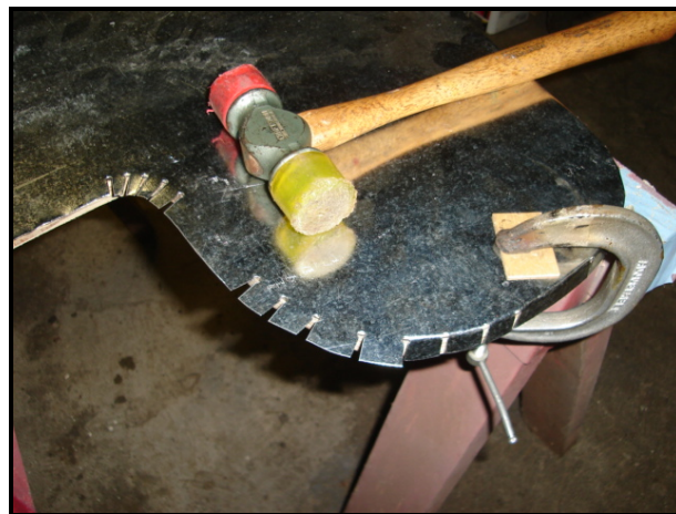
Forming the Flange (Note the Slots in the Flange)
