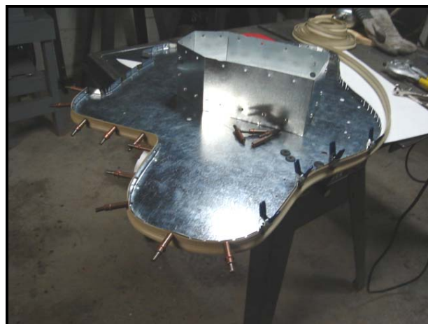
Installing the Seal
