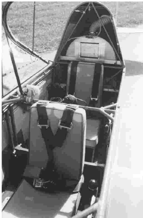
The rear view of the cockpit shows the 5 gallon auxiliary fuel tank mounted behind the pilot, and some nice detail of the seat cushions.
