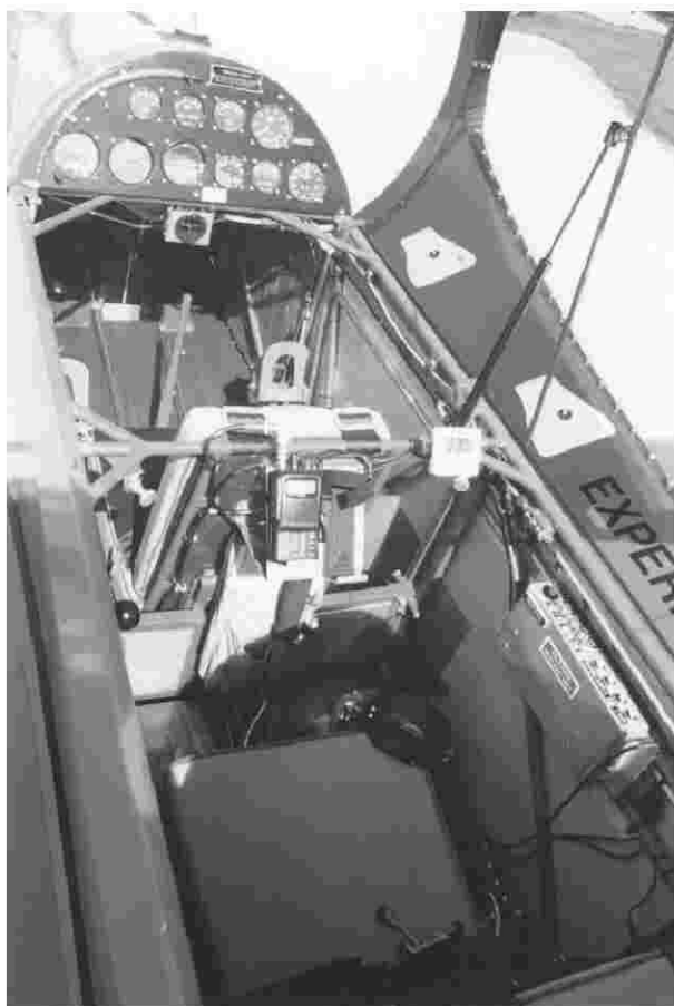
This view of the cockpit looking forward shows several interesting goodies. The first is the toe brakes on the rear rudder pedals. The second is electrical system control module on the RH side of the rear cockpit that contains all the switches and circuit breakers. Also note the neat layout of the instrument panel and the canopy support.
