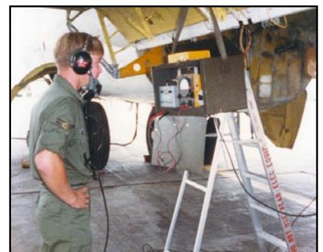
*Above, a 19-year old Kerry Fores performs a Critical Circuits Check on a B-52 prior to a weapons loading operation. Minot, 1983.*
