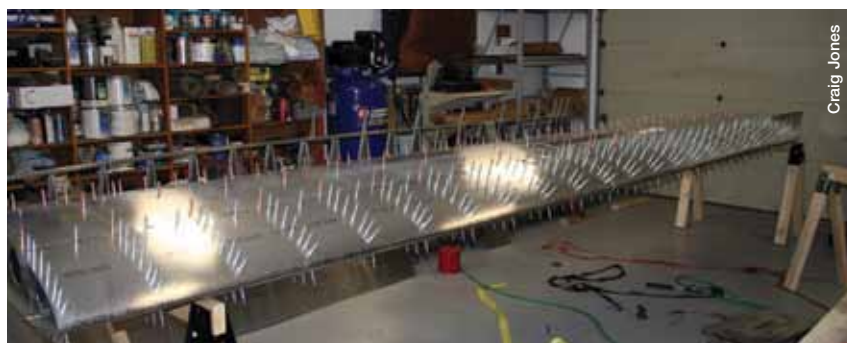
Part of the price for a 24-to-1 glide ratio is building an airplane with a 45-foot, 8-inch-span wing. Each wing has 28 laser-cut ribs, each spaced a few inches apart.
