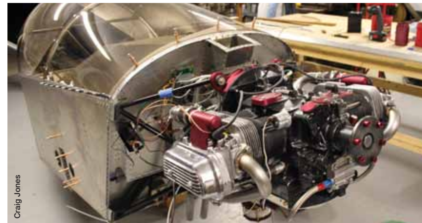
Choosing the Volkswagen-based AeroVee engine was a natural for Craig, since he was familiar with them from his early auto-racing days.
