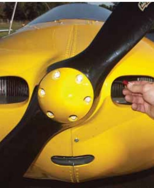
The demonstrator Waix is powered by an 80-hp AeroVee engine; using this flexible dipstick, you can check for oil without having to open any cowl doors.
