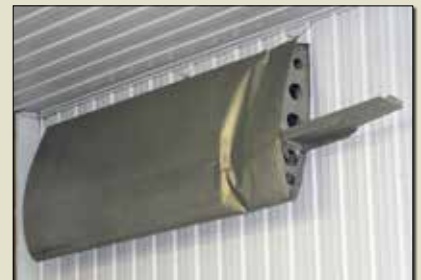
Trophies of static load testing adorn the prototype shop wall. This Sonex wing failed well above design loads.
