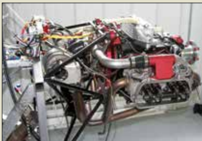
The new turbocharger adds horsepower to the AeroVee engine in a clean, spacious installation. Shown here in a test stand, it is currently flying in a factory Sonex.
