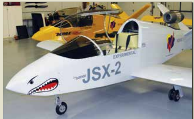
The SubSonex kit includes the PBS TJ-100 turbojet engine, retractable gear, and a BRS full-aircraft parachute recovery system.
