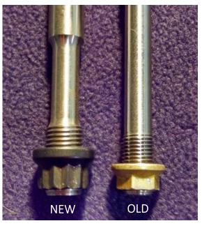
Larger 7/16" through-bolts, studs and nuts (left) provide more torque strength to eliminate the possibility of thread stretching and case fretting over time.
