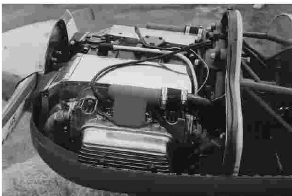
LH view of the engine installation. Note how tightly the engine is mounted to the firewall.
