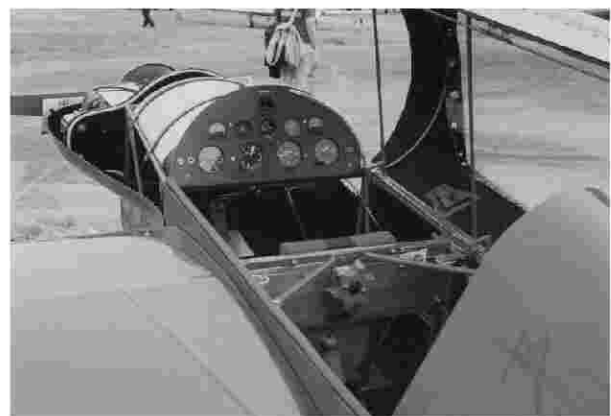
The cockpit and instrument panel. The large knob on the spar carry-thru is the elevator trim.
