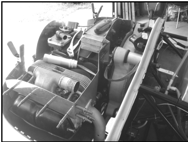
Initial Cooling Baffle Fit Up
