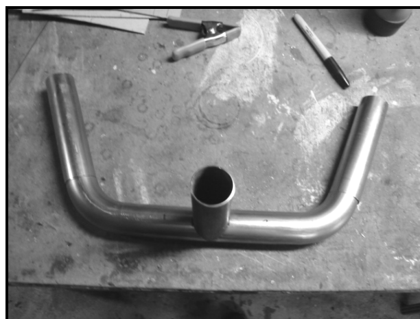
Intake Manifold Ready for Welding
