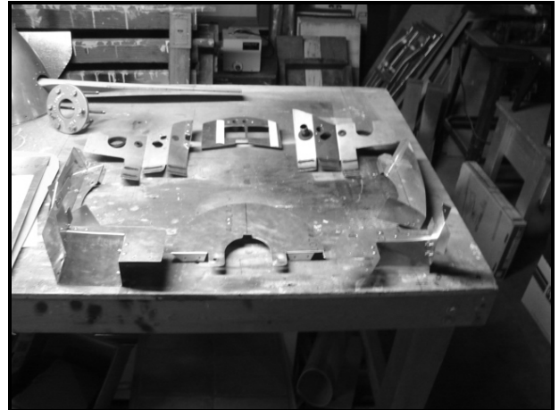
Finished Baffles Before the Silicone Seals
