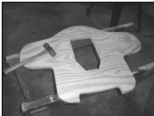
Form Block with the Box Cutout.
