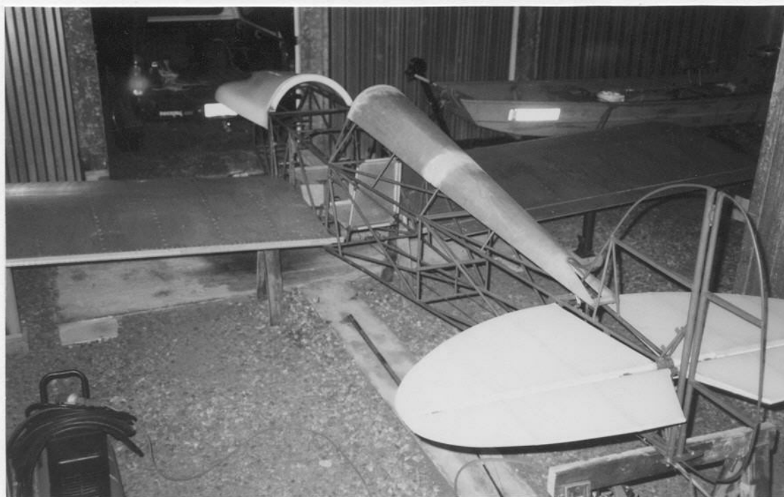
January 1997 – Finished Welding and Test Fit Parts
