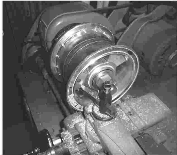
Machining the Mounting Surface
