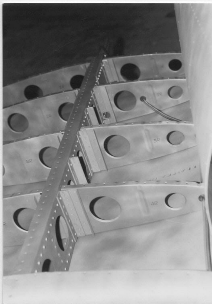
Photo 1 - Front Ribs to Main Spar
